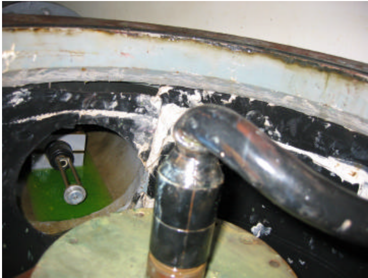
Fig. 3: Bent cable providing power and data control to the transducer heads. Note the velocimeter in the background. The cavity was filled with hard styrofoam in St. John's July 19, 2003 to reduce resonance and ringing within the well.
