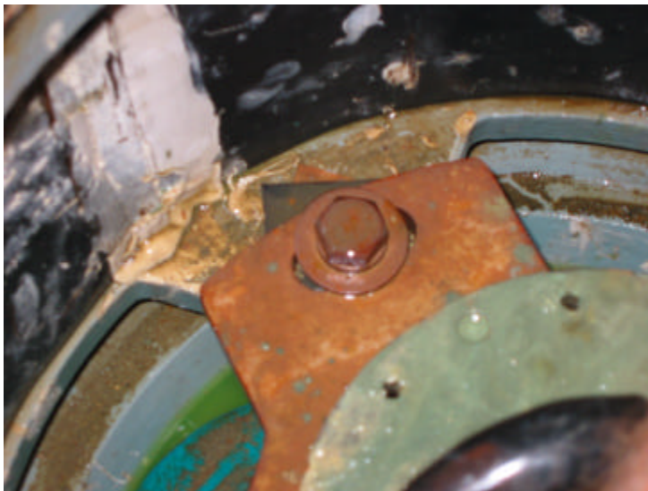
Fig. 2: Mounting of the transducer plate to the ship's hull. Note the this strip of rubber that is probably insufficient to acoustically insulate the ship's vibrations from the transducer heads.
